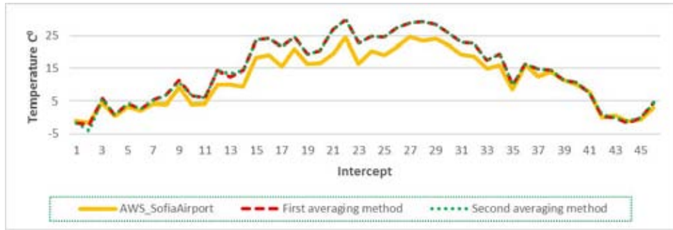
Fig. 2. Comparing AWS Sofia Airport in-situ near-surface temperature observations with averaged MODIS LST observations after the 1 st and 2 nd method for 2013
